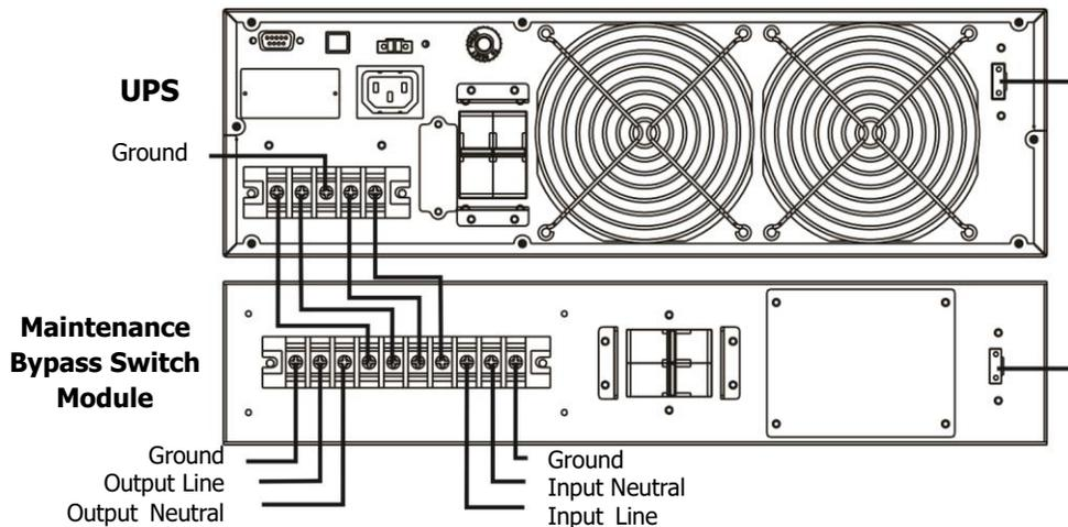
**NOTE :** Make sure that the wires are connected tightly with the terminals.
